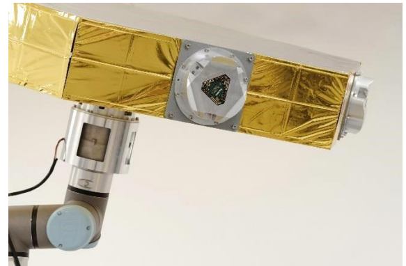
Robot manipulator provided with SIROM as end effector handling a mirror tile.
