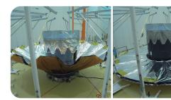
12 identical frames that deploy simultaneously and that hold two thermal covers arranged in parallel.
