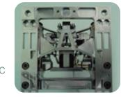
M2M is designed to operate in a temperature range that goes up to 110 K with a very good thermal stability and, equally, it is able to stand the launching loads without hold down.
