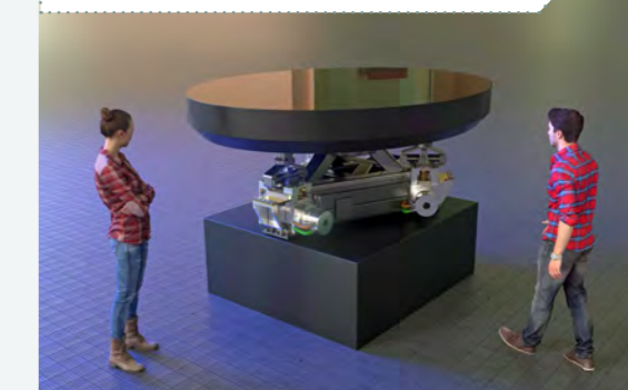
Artist's impression of the M5 mirror of the European Large Telescope (ELT).
