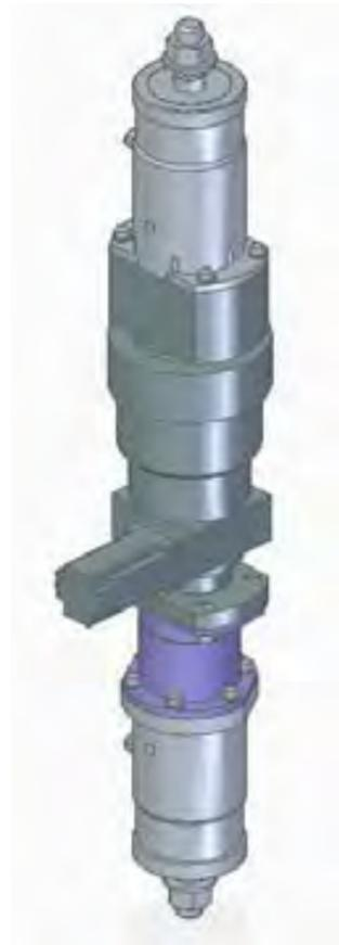
Hybrid actuator prototype. | NEReA non-explosive release actuator.
