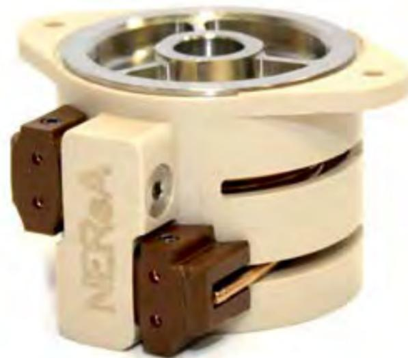
**Hybrid actuator prototype** for the rapid guiding movement and alignment of secondary mirrors in large ground-based telescopes. This development is based on a conventional electromechanical actuator to perform the alignment with and over a large range, in addition to another electric piece that provides the rapid movement.
