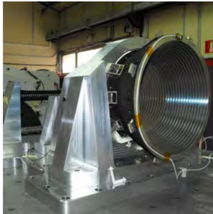
Band feed horn antenna assembly, in aluminium alloy, during random vibration test.
