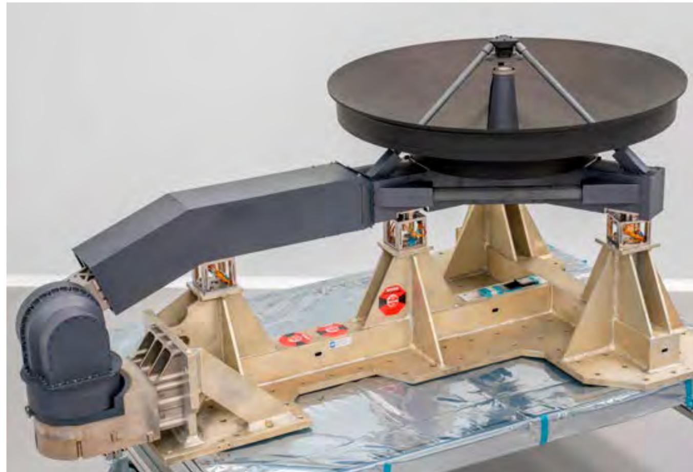
Solar Orbiter High Gain Antenna Gimbal (HGAG).
